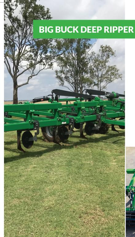
The Gessner Big Buck is a proven performer and one of Australia's most trusted deep ripping implements. Manufactured from premium 350 grade steel, the Big Buck deep ripper is both structurally robust and versatile.
