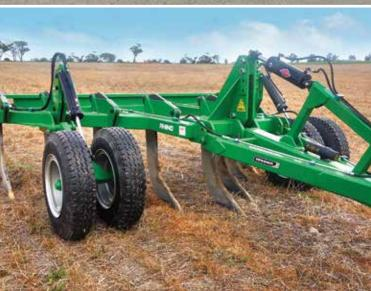
Experience the ultimate in deep tillage solutions with Gessner's Rhino Ripper. Featuring an industry leading 250mm x 150mm x 10mm main beam and high tensile tines and tungsten wear-parts, the Rhino Ripper is the deepest commercially made ripper on the market with a maximum ripping depth of 900mm.
